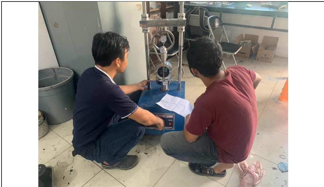
Gambar A.12 Proses perhitungan marshall
