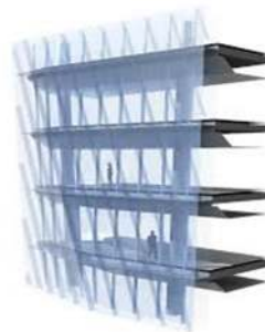
Gambar 5.14. Double Skin Façade (Sumber : www.modlar.com/foster-fasade )
