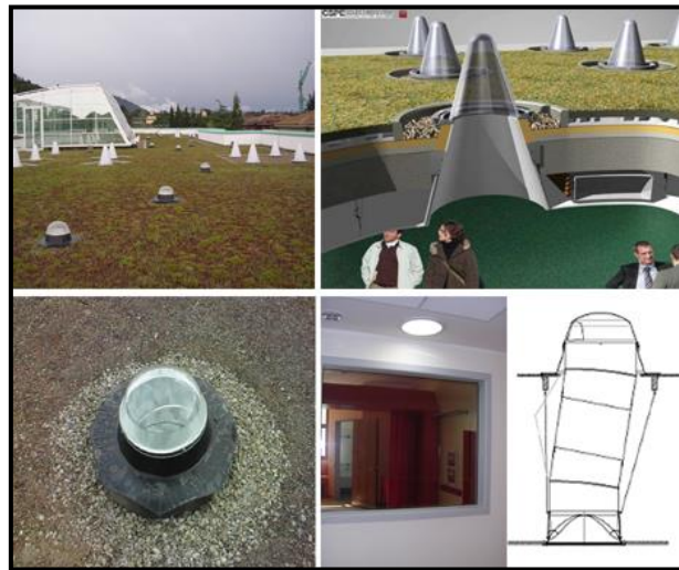
Gambar 3.42 Sun Pipes And Light Ducts
