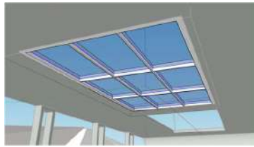
Gambar 5.2 System Skylight Sumber: https://Analisa Penulis,2024
